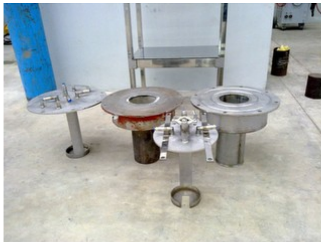
These are ‘bomb reactors’ likely used to convert uranium compounds into uranium metal for bomb or reactor fuel (DVB)
