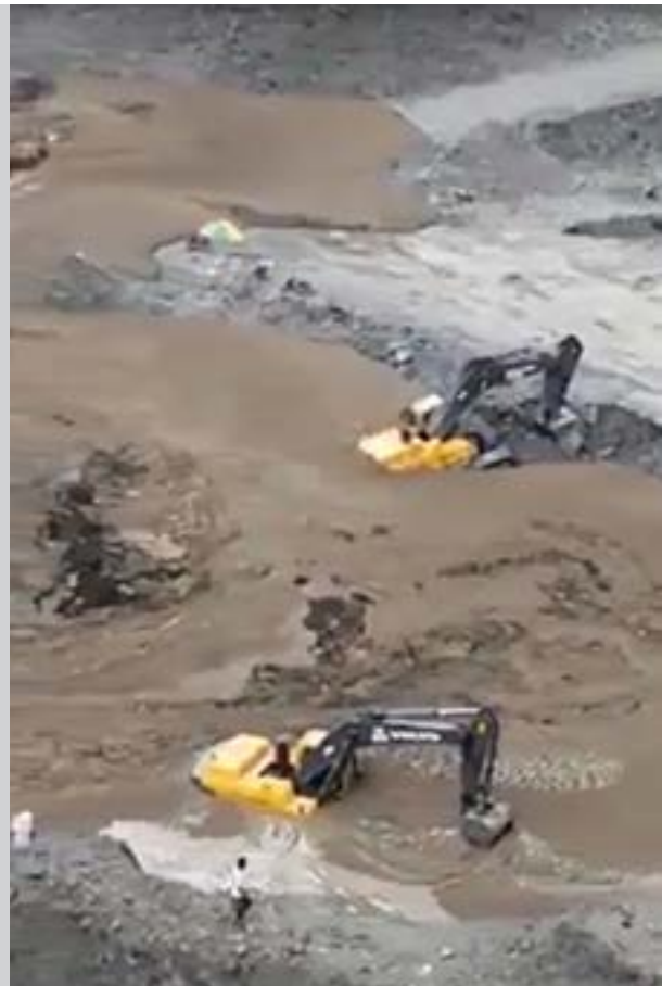
Stills from a video of a massive mud slide that took place at the Myat Yamon Kaday (#2) mine in April 2015. Local residents put the death toll at 30 to 60 people. The accident is said to have occurred due to the company's persistent dumping of tailings on a bed of liquid mud above the mine. The waste then shifted and flooded into the crater, engulfing workers and machines in its path.
